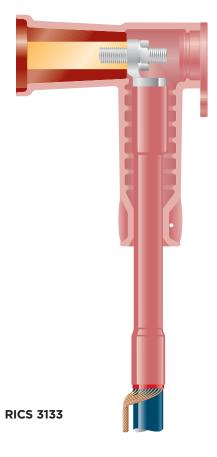
This insulated adapter provides perfect sealing, electrical insulation and an electrical connection between all Raychem terminations and SF<sub>6</sub>-insulated switchgear up to 12 kV. It is designed to fit bushing profiles according to EN 50181 type C.
